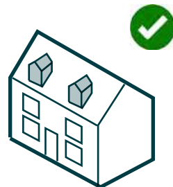
Loft conversion incorporating gable dormers.
